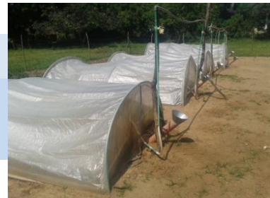
Right Photo: A typical Flexi-Biogas System (Pwani University Flexi Biogas Unit)
